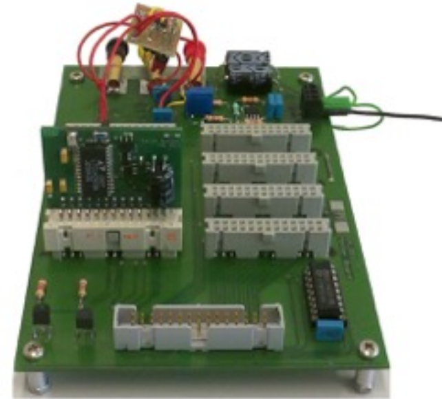
8-channel Implementation of Analog CS
